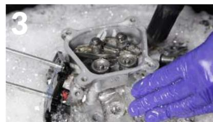
3 Heated to 42°C, the microbes become active in the ROWash Degreasing solution and eat the oil and grease turning them into harmless CO<sub>2</sub> and water - effectively recycling the fluid.
