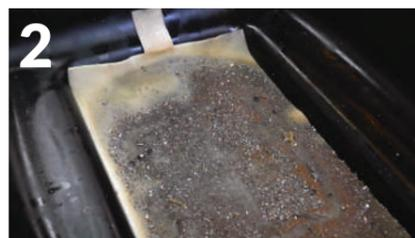
2 The Filter Mat is the KEY to the system - it contains 200 million oil-eating microbes and traps particles down to 50 micron.
