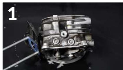
1 Oil and grease are washed off the dirty part and flow through the Microbial Filter Mat in the sink into the ROWasher tank.
