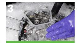
active in the ROwash Degreasing solution and eat the oil and grease turning them into harmless CO<sup>2</sup> and water – effectively recycling the fluid
