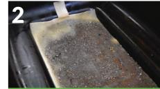
The Filter Mat is the KEY to the system - it contains 200 million oil eating microbes and traps particles down to 50 micron.
