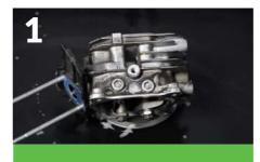
Oil and grease are washed off the dirty part and flow through the Microbial Filter Mat in the sink into the ROwasher tank.
