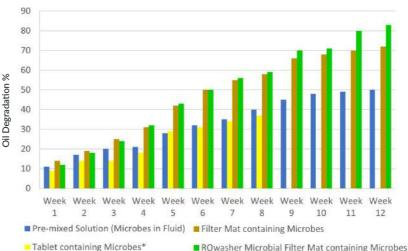
The figure shows the oil degradation rate in the ROwasher over 12 weeks compared with competitor bioremediating parts washers.
